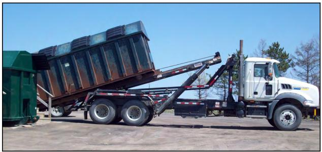
Photo 4: Pulling Recycling Roll-off
