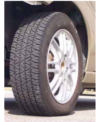
Tire at 16 psi (50% recommended pressure)
