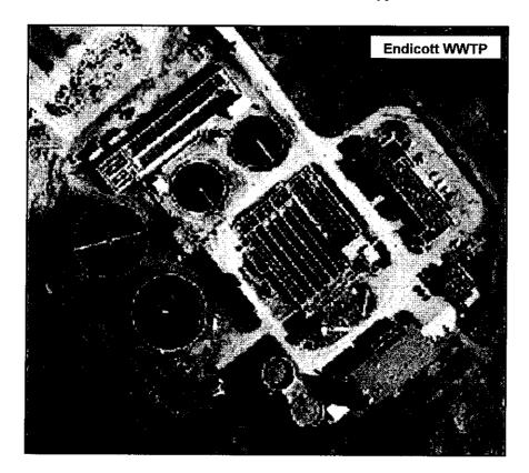
The Endicott WWTP has a permitted maximum month flow of 10 mgd; the current average annual flow is 8.3 mgd with an associated maximum month flow of 14 mgd. The original plant was constructed in 1966 and included primary treatment. In 1973, the plant was upgraded to include secondary treatment with trickling filters. In 2002, the plant was again upgraded with new plastic media biotowers (trickling filters), solids contact tank, and additional secondary clarifiers.
